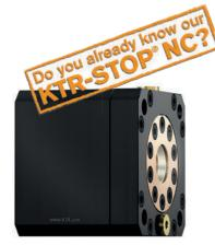
The KTR-STOP® NC series is a passive clamping and braking system. It serves for generating a clamping/braking force respectively a clamping/braking torque on a cylindrical piston rod or shaft. This results in a delay of the rotary motion respectively keeping at standstill. For further details please refer to page 146/147.
