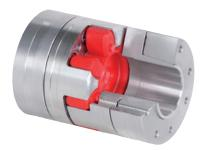
**ROTEX® GS** is a three-part, axial plug-in coupling backlash-free under prestress. It is convincing even with critical applications by its backlash-free power transmission, its stiffness which is each adapted to the application and its optimum damping of vibrations. This principle of installation offers significant options of assembly optimizing the assembly times in production.
